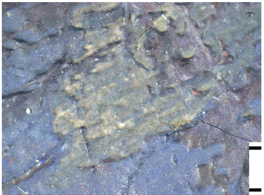
Fig. 10 In one place where overlying paint was not applied, a thin underlying layer can be discerned, microscopic photograph (M = 1 mm)
