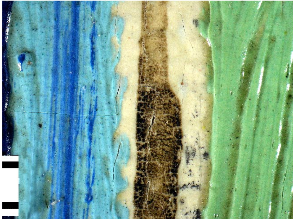
Fig. 13 Brown India ink drawing and traces of pencil, microscopic photograph (M = 1 mm)
