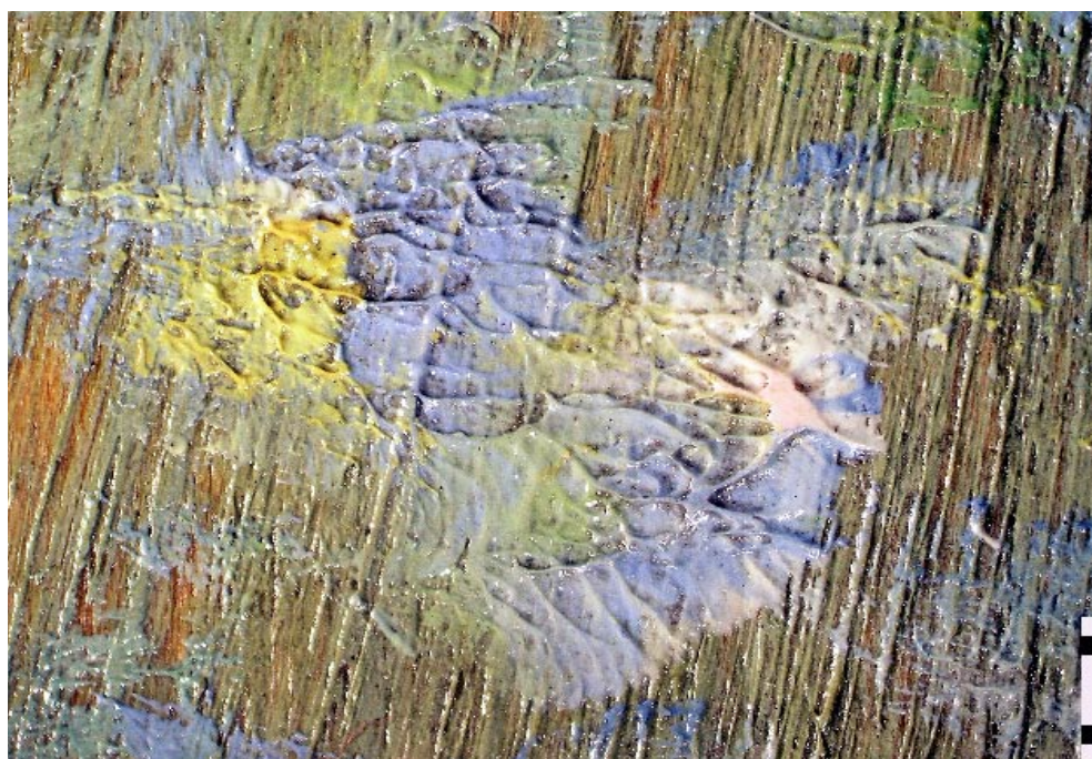
Fig. 10 The surface structure of the paint application, microscopic photograph (M = 1 mm)
