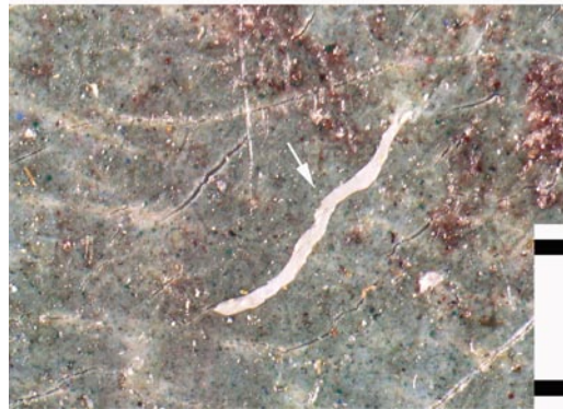
Fig. 11 Paint or ground which has penetrated from underlying layers through the network of early shrinkage cracks, microscopic photograph (M = 1 mm)
