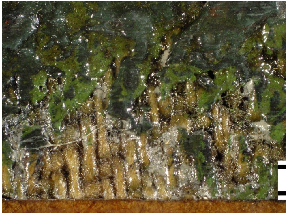
Fig. 5 Twill-weave canvas, microscopic photograph (M = 1 mm)
