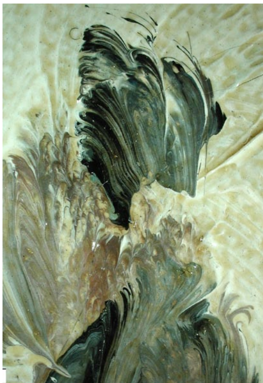
Fig. 11 Wet-in-wet paint application with black pigment, microscopic photograph (M = 1 mm)
